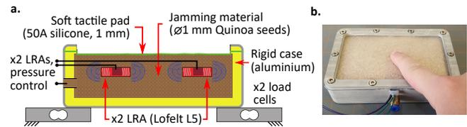
Fig. 1. a: Schematic view of the interface. b: Working prototype interface
